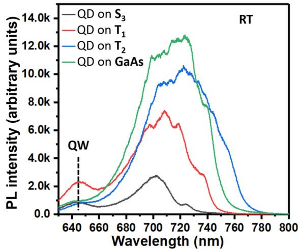
FIG. 6. RT-PL spectra of the InP QDs grown on the native GaAs and the different GaAs/Si templates pumped at  $2.5 \mu\text{W}$ . PL intensity of the QDs on the GaAs/Si templates increased with the decrease in defect density.
