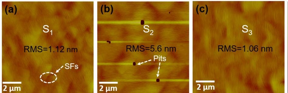
**FIG. 2.**  $10 \times 10 \mu\text{m}^2$  AFM images of sample (a)  $S_1$  with SFs, (b)  $S_2$  with pits, and (c)  $S_3$  with smooth surface. The RMS values for these three samples are 1.12, 5.6, and 1.06 nm, respectively. The color scale is 30 nm.
