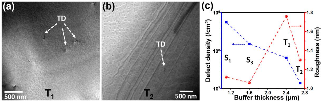
**FIG. 4.** PV-TEM images of samples (a)  $T_1$  and (b)  $T_2$ . (c) Surface roughness and defect density of the GaAs/Si templates vs buffer thicknesses. Defect density decreased from  $5.8 \times 10^8$  ( $S_1$ ) to  $1.4 \times 10^7$   $\text{cm}^{-2}$  ( $T_2$ ), and  $T_2$  has a smooth surface with an RMS value of 1.3 nm.
