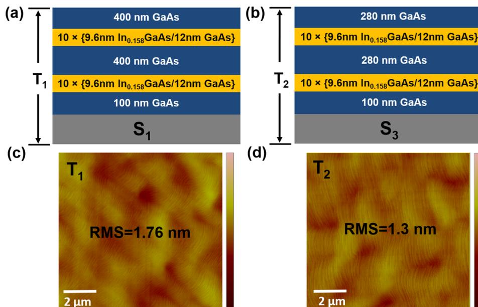
**FIG. 3.** Schematic diagrams of samples (a)  $T_1$  and (b)  $T_2$ . Both  $T_1$  and  $T_2$  contain two sets of 10 periods of 9.6 nm  $\text{In}_{0.158}\text{GaAs}/12$  nm GaAs SLSs, and the spacer thicknesses in  $T_1$  and  $T_2$  are 400 and 280 nm, respectively.  $10 \times 10 \mu\text{m}^2$  AFM images of sample (c)  $T_1$  and (d)  $T_2$ . RMS values for these two samples are 1.76 and 1.3 nm, respectively. The color scale is 30 nm.
