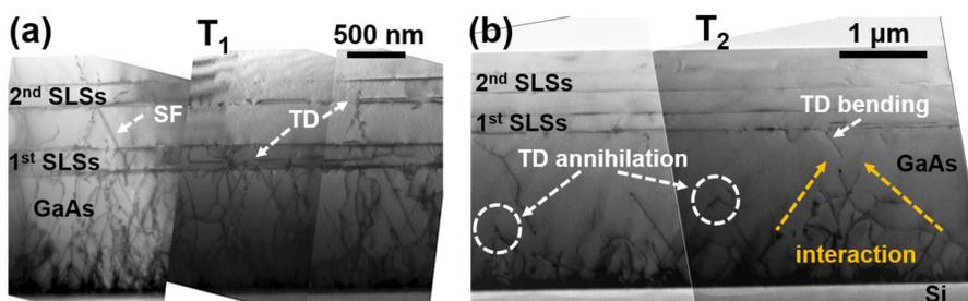
**FIG. 5.** X-TEM images of samples (a)  $T_1$  and (b)  $T_2$ , respectively. Some TDs and SFs could not be trapped by second SLSs in  $T_1$ , while the interaction of defects took place obviously in GaAs epilayer of  $T_2$  due to the higher annealing temperature.
