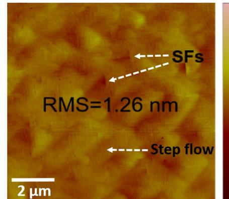
FIG. 1.  $10 \times 10 \mu\text{m}^2$  AFM image of a 1  $\mu\text{m}$ -thick GaAs/Si template with step flow and SFs. The RMS value is 1.26 nm. The color scale is 30 nm.
